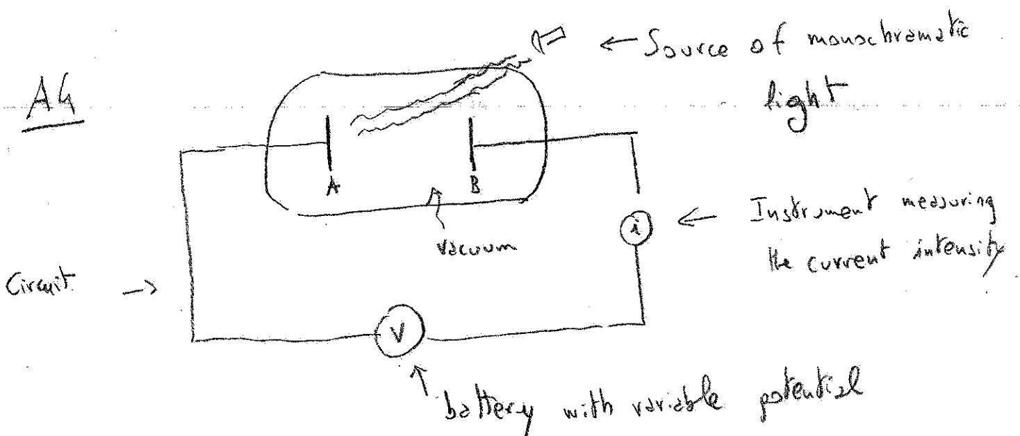
The stopping potential  $V_s$  is the potential the battery needs to provide to stop the current flowing in the circuit. This means that electrons are stopped before reaching plate B because the potential energy is bigger than their initial kinetic energy - this kinetic energy depends on the energy of each incident photons ( $E_p = hf$ ) and thus is related to the frequency, and not to the intensity (which measures the number of photons in the beam).
